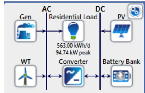
Fig. 1. Design of the proposed hybrid micro-power system
