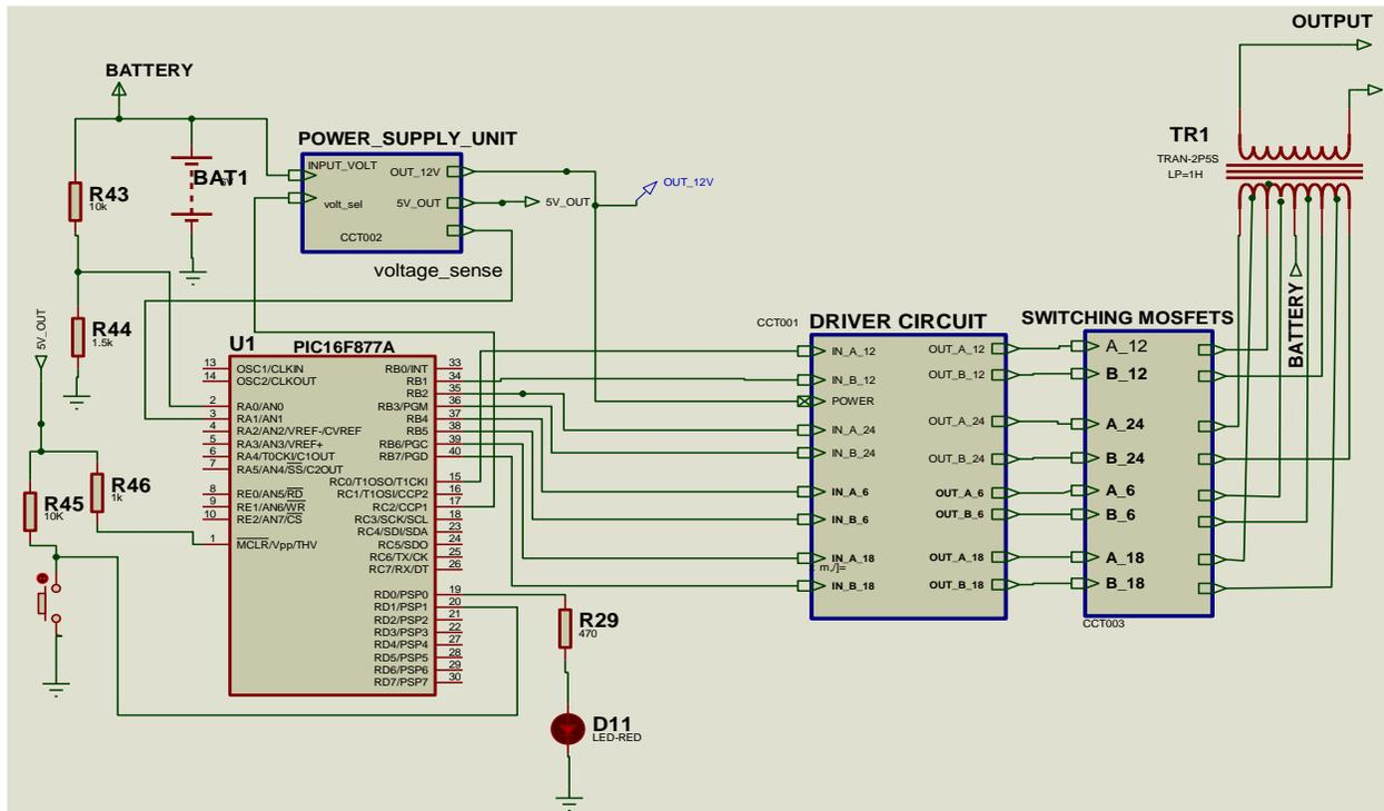
Fig. 2. The Overall Schematic Diagram of the Power Inverter System.
