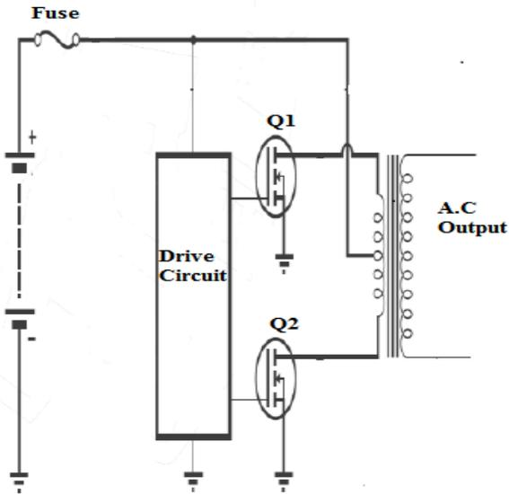
Fig. 1. Push-Pull Inverter Circuit.
