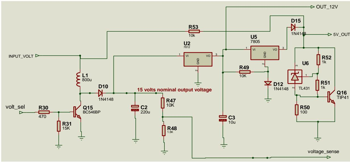
Fig. 3. Schematic Diagram of the Power Schematic diagram of the DC to DC converter circuit.
