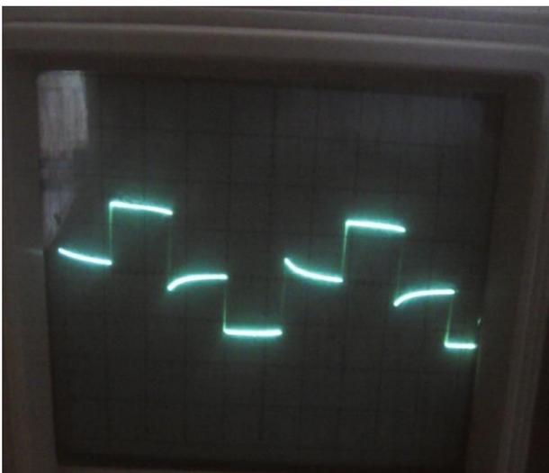
Fig. 6. Sample Output Waveform of the Inverter Circuit.
