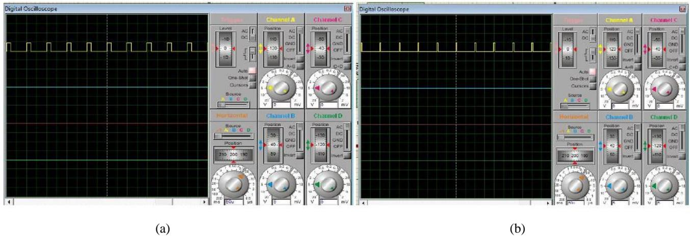
Fig. 4. The Dc to Dc Converter pwm Control Signal for Battery voltages of (a) 6 V and (b) 12 V.
