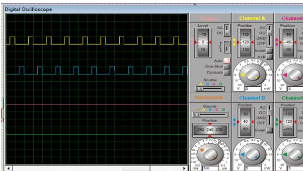
Fig. 5. The A Sample of the Inverter Drive Signal at the i/o pin of the Microcontrollers.
