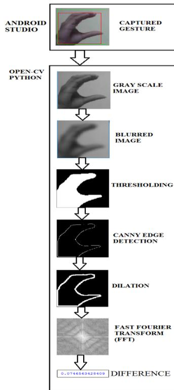
Fig 7. Real-time capturing of gesture and stepwise image processing.
