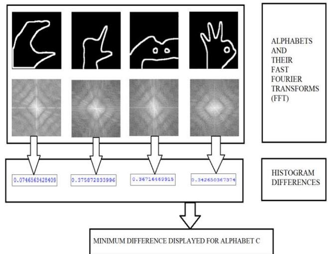
Fig. 9. Result after comparing the difference of testing image C with training database images.
